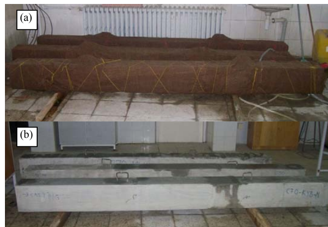
Fig. 1 Curing methods applied to the samples (a): moisture cure, (b): air cure
