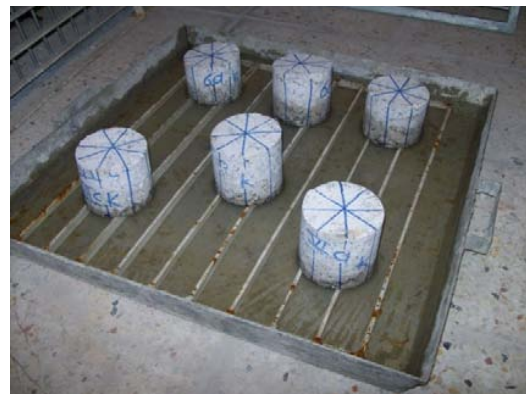
Fig. 4 Capillary water absorption experiment
