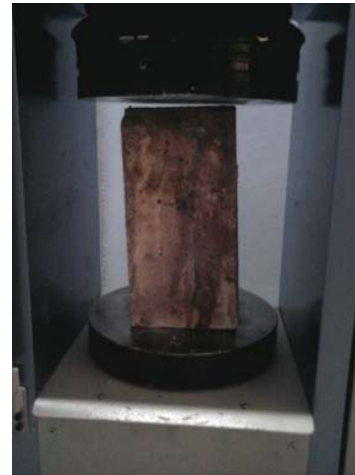
Fig. 6 A corroded column specimen before compressive testing
