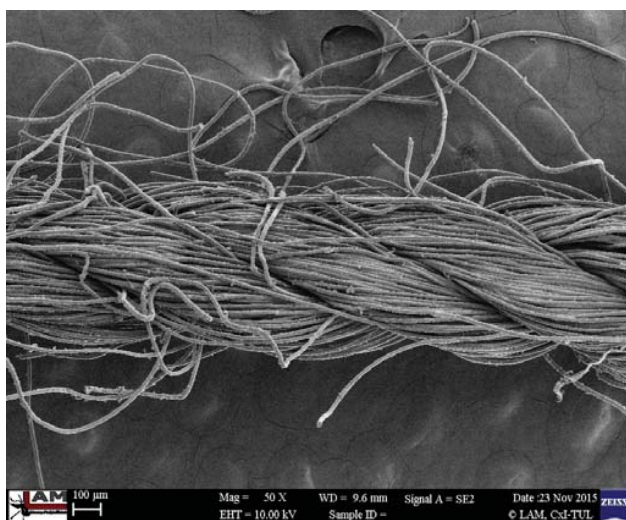
Fig. 10 SEM image of sample 3B after sewing (4000r/min)
