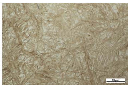
Fig. 1 Optical microscopy of sample A at magnification of 100x – etched or before immersion into 1.0 M NaCl solution
