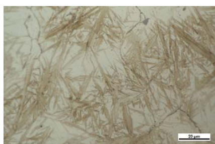
Fig. 2 Optical microscopy of sample B at magnification of 100x – etched or before immersion into 1.0M NaCl solution
