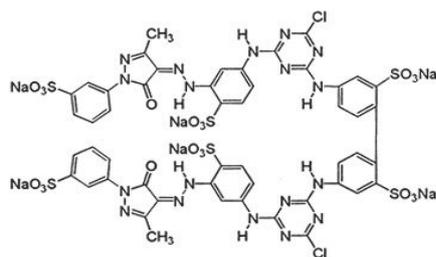
Fig. 2 Molecular structure of reactive dye named Reactive yellow 105(C<sub>50</sub>H<sub>32</sub>Cl<sub>2</sub>N<sub>18</sub>Na<sub>6</sub>O<sub>20</sub>S<sub>6</sub>)
