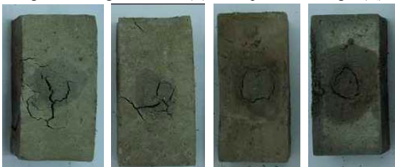
Non-baked specimens: severely damaged during tests
