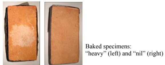
Fig. 11 Efflorescence test results
