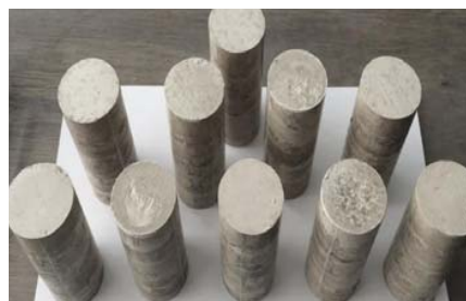
Fig. 3 prepared specimens for UCS test
