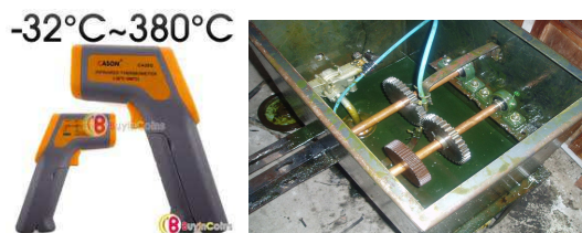
Fig. 1 Illustrates Laser Gun Temperature (left) test rig with load (right)
