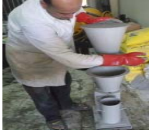
Fig. 3 Compaction Factor Measurement of Fresh Geopolymer Concrete
