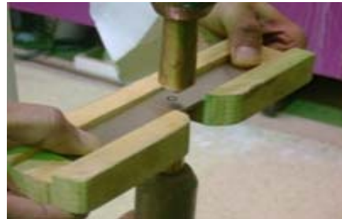
Fig 2 Spot welding specimen holder
