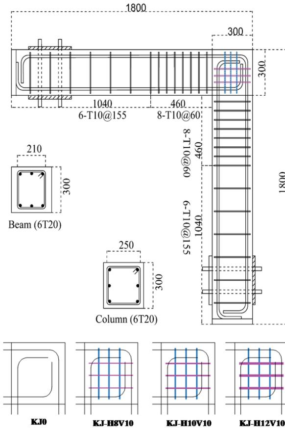
Fig. 1 Geometry and reinforcement layout of specimens
