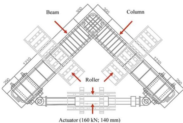
Fig. 2 Test setup
