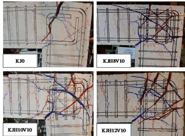
Fig. 5 Cracking patterns of specimens
