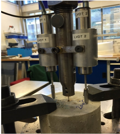
Fig. 2 Single fibre pull-out test setup
