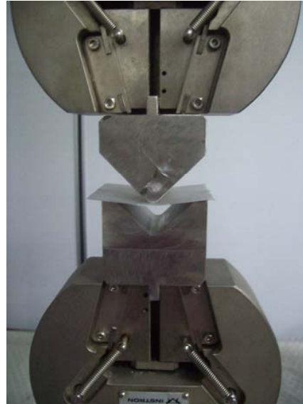
Fig. 2 Experimental set-up for V-bending process
