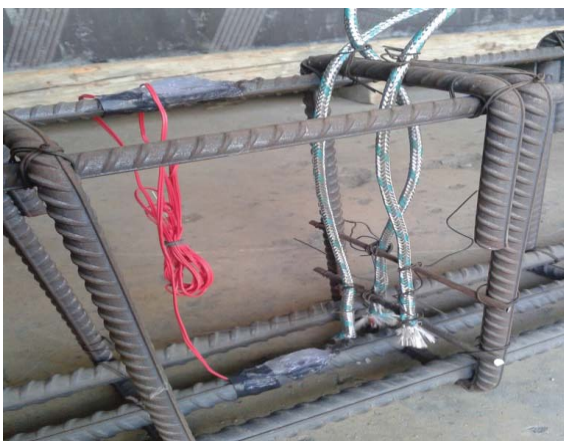
Fig. 2 Location of thermocouples at beams midspan
