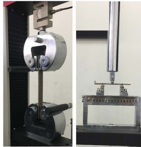
Fig. 4 Tensile and flexural testing of developed composites on UTM machine
