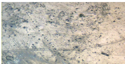
Fig. 26 Micrograph of 25% groundnut shell filler
