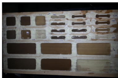
Fig. 4 Mould filled with CBRPC samples
