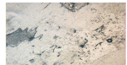
Fig. 23 Micrograph of 20% groundnut shell filler
