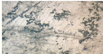
Fig. 22 Micrograph of 20% cow bone filler
