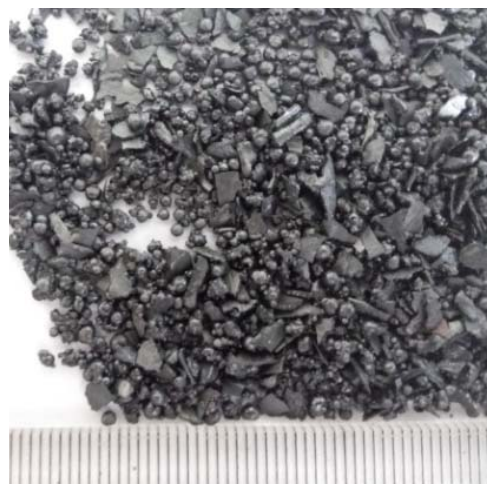
Fig. 2 Particle morphology of granulated slag
