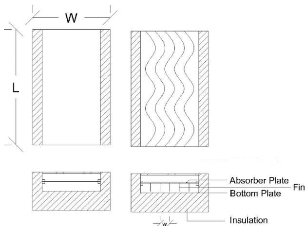
Fig. 1 Solar air heater with wavy fin absorber
