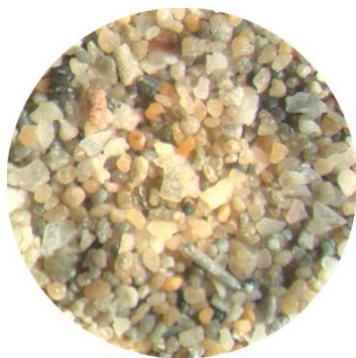
Fig. 1 Microscopic image of Bushehr calcareous sand
