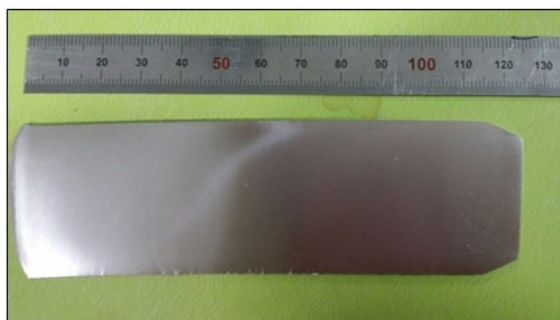
Fig. 6 Appearance of hot rolled sheet of nonflammable AZ91D alloy obtained at 400°C through 5 passes. Final thickness was 0.9mm
