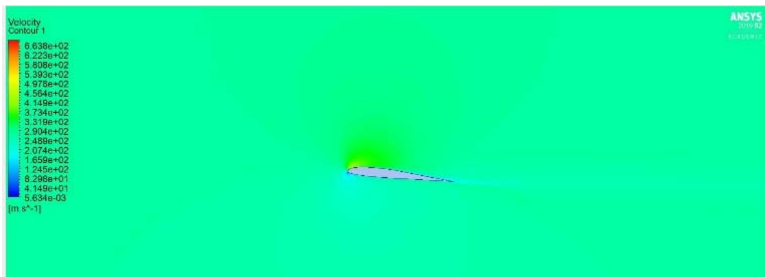
Fig. 12 (a) Velocity Contour of SD7003 in pre-stall
