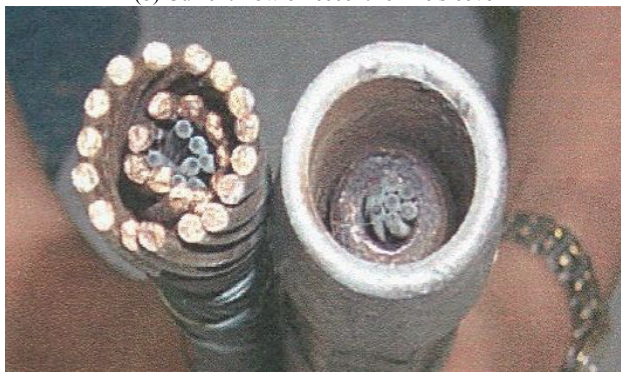
Fig. 2 Line Sleeve current flow and broken sleeve
