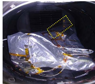
Fig. 5. Heat pipe subsystem in a vacuum chamber.
