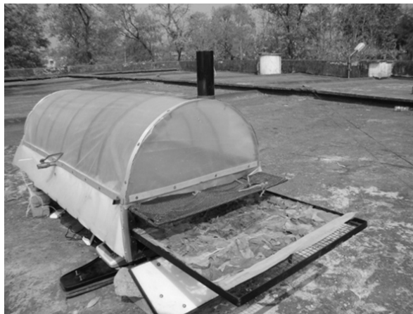
Fig. 1 Experimental set-up of spinach drying in solar tunnel dryer (STD)
