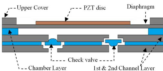
Fig. 3 The AA section view for the micro pump
