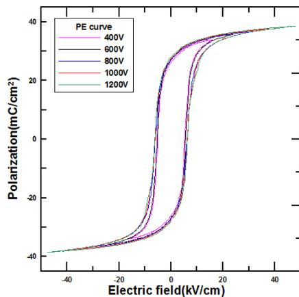
Fig. 6 P-E hysteresis curves of the Piezoelectric disc
