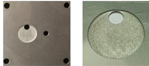
Fig. 4 The fabricated stainless steel channel layer
