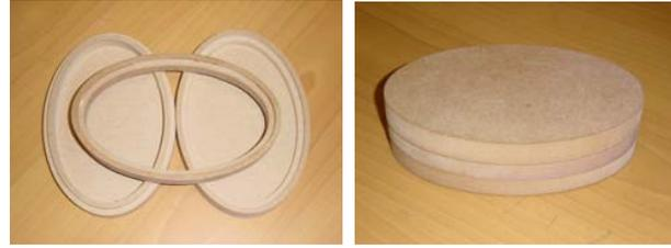
Fig. 10 A MDF-board elliptic box
