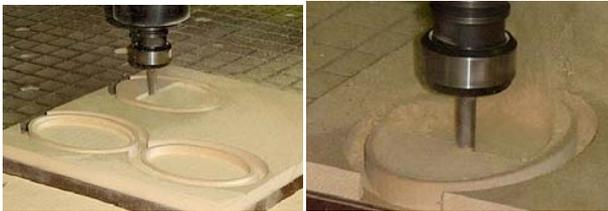
Fig. 9 MDF-board (Medium Density Fiberboard) machining of ellipses
