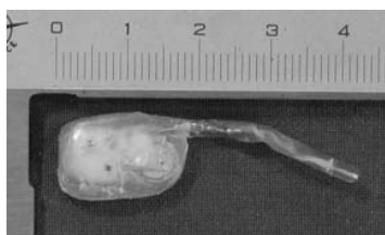
Fig. 2 The wireless intraoral pH telemeter
