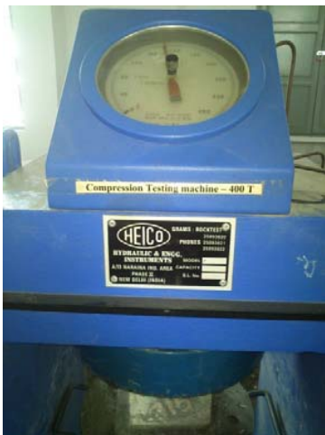
Fig. 6 Compressive strength Test
