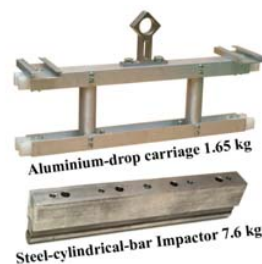
Fig. 1 Aluminium-drop carriage and steel cylindrical impactor
