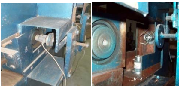
Fig. 7 Load cells attached with the roller bearings
