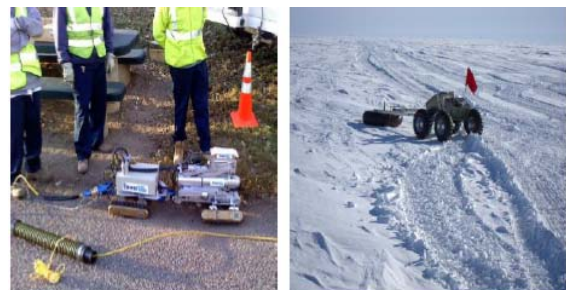
Fig. 4 Sewervue [15] and Yeti Robot [16] in operation
