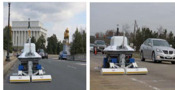
Fig. 3 Operation of GPR bridge deck assessment robot [14]
