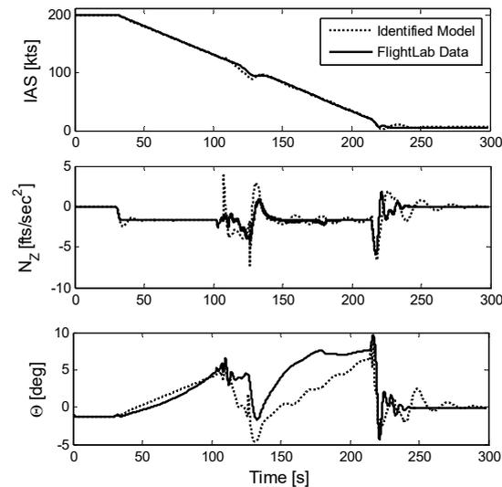
Fig. 6 Comparison between identified model outputs and simulated flight data for conversion from aircraft to helicopter: rigid body dynamics
