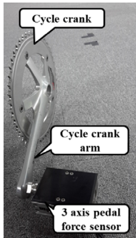
Fig. 1 Three-axis Pedal Force Measurement Sensor installed Device
