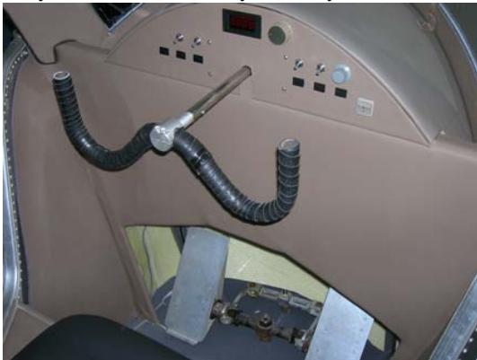
Fig. 6 Real cockpit with control loading system
