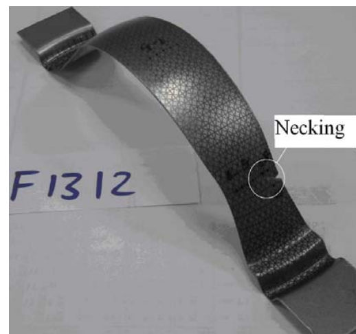
(b) 30×180 mm 2 sheet metal specimen
