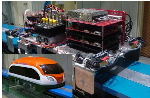
Fig. 9 The miniature maglev using hybrid magnets
