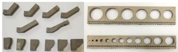
Fig. 12 Fabricated overhang test specimens by EBM
