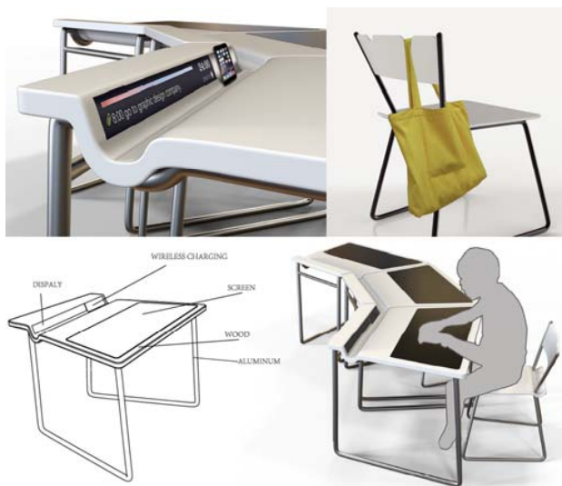
Fig. 13 The Wave, main features
