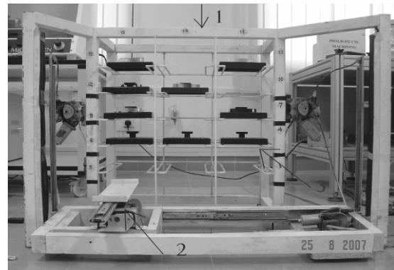
Fig. 3 Developed AS/RS structure
