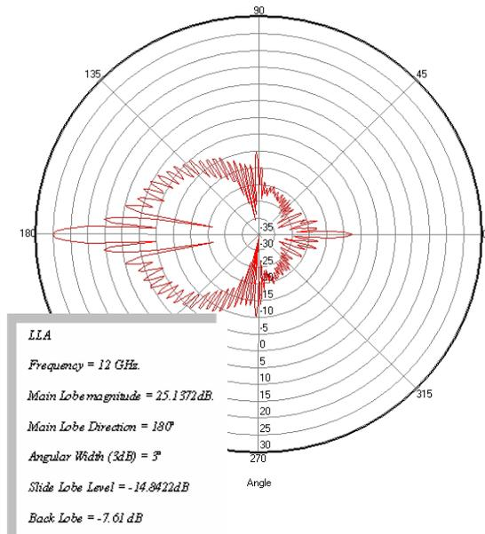
Fig. 10 The Radiation pattern of the LLA
