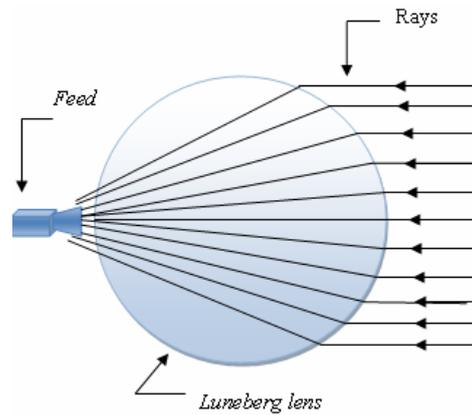
Fig. 4 The Conventional Luneberg lens antenna (CLLA)
