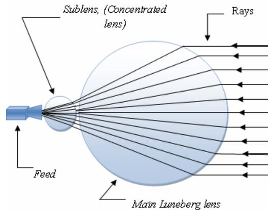
Fig. 5 Luneberg lens with Concentrating lens antenna
