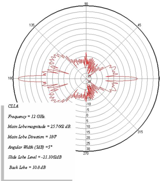
Fig. 11 The Radiation pattern of the CLLA
