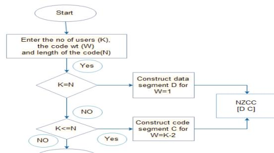
Fig. 1 Flow chart for NZCC code family construction
