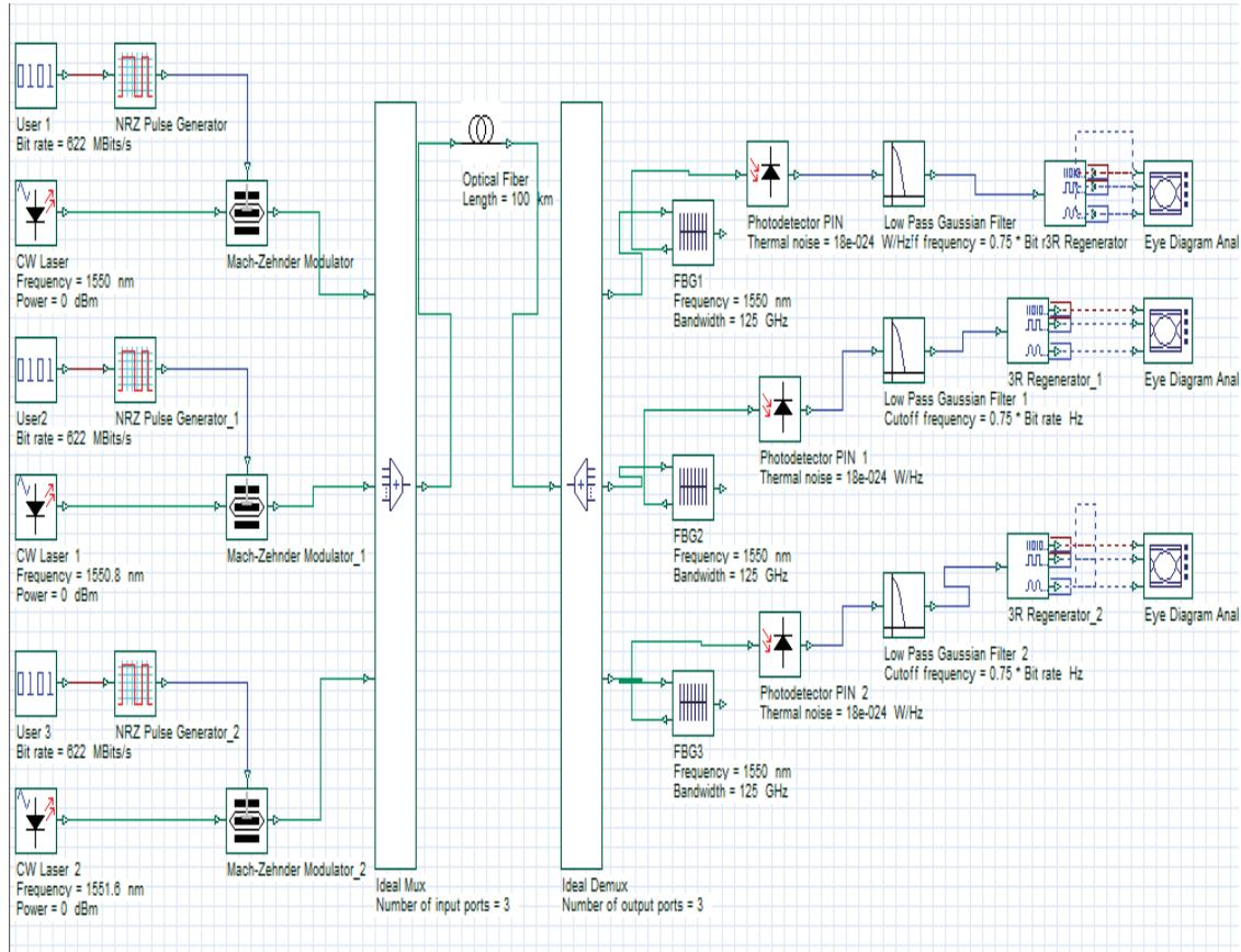
Fig. 2 Simulation circuit for 3 users [19]
