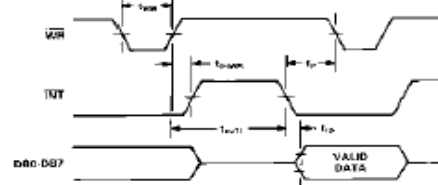
Fig. 5: AD7821 stand-alone operation
