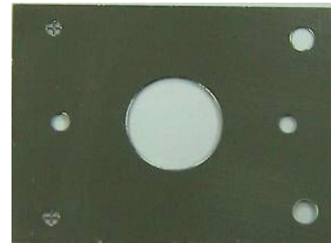
Fig. 7 The fabricated nickel chamber plate I
