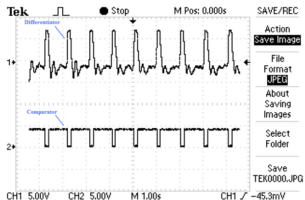
Fig.18 Heart beat signal obtained from differentiator and comparator
