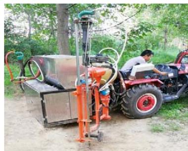
Fig. 5 Experimental prototype of orchard gas explosion subsoiling and fertilizer injection machine
