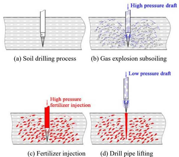
Fig. 2 Working process of orchard gas explosion subsoiling and fertilizer injection machine
