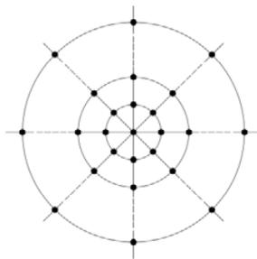
Fig. 7 Schematic diagram of soil compaction test points
