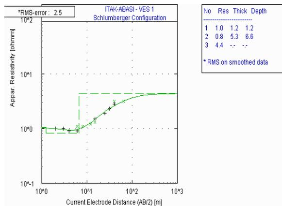
Fig. 1 Geoelectric Sounding Curve Obtained from VES 1
