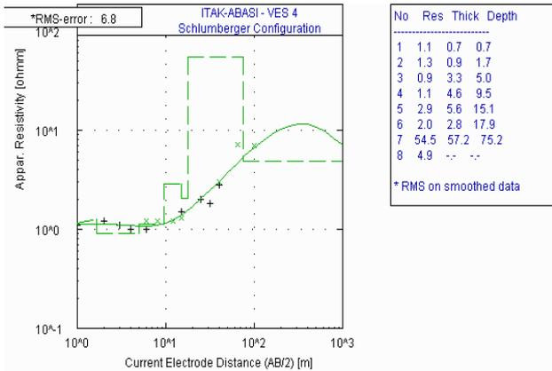
Fig. 4 Geoelectric Sounding Curves Obtained from VES 4
