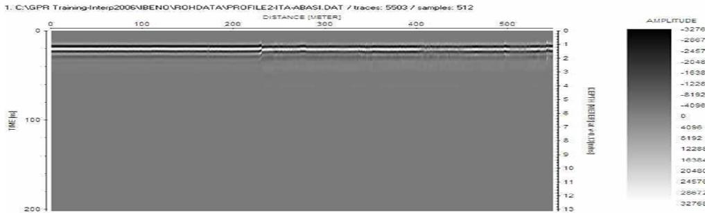
Fig. 11 Profile 2 Raw Field GPR Data (Itak-Abasi)
