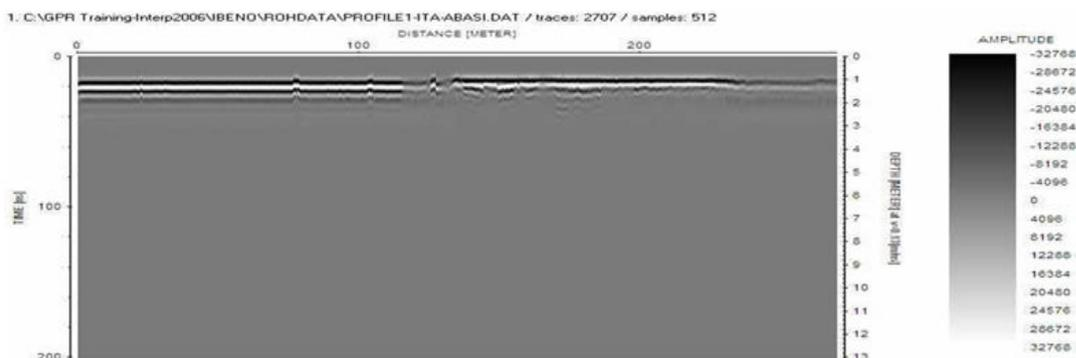
Fig. 9 Profile 1 Raw Field GPR Data (Itak-Abasi)
