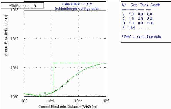
Fig. 5 Geoelectric Sounding Curve Obtained from VES 5
