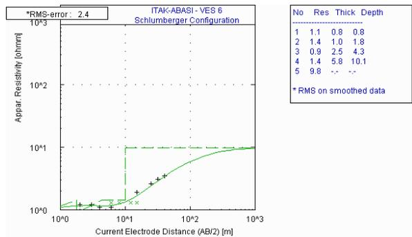
Fig. 6 Geoelectric Sounding Curves Obtained from VES 6
