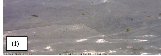
Fig. 4 (a) Control sample (b) Exposed 1 st month. (c) Exposed 2 nd month (d) Exposed 3 rd month. (e) Rougher surface at 4 th month exposure (f) Fragmenting started in sample at 5 th month
