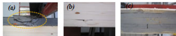
Fig. 6 Failure modes (a) failure of UHPFRC plank, (b) failure of timber beams in tensile (c) failure of CFRP and collage
