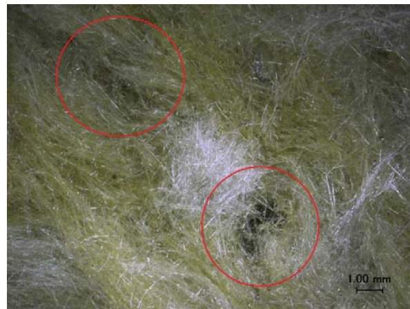
Fig. 15 Curling of mineral fibers with discontinuities in the center
