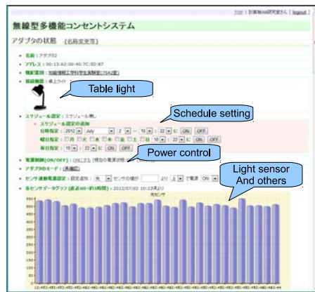
Fig. 6. Screen shot of a web browser displaying sensors graph and control
